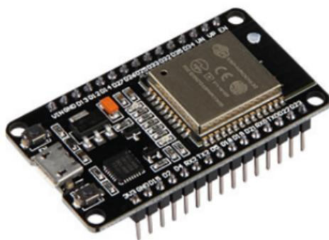
Figure: ESP32 on a dev board
